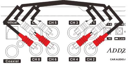
1: Input the machine with RCA low level signal line;
